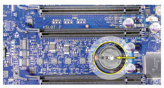
Warning: Installing the battery incorrectly may cause an explosion. Be sure the battery's positive and negative sides are correctly oriented in the holder. Use only the same type of battery or an equivalent recommended by the manufacturer of the original.
